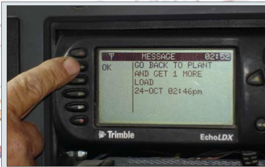
◀ *Trimble's telematics solution has an available in-cab monitor to provide truck and equipment operators with detailed information, including whether more materials must be picked up.*
